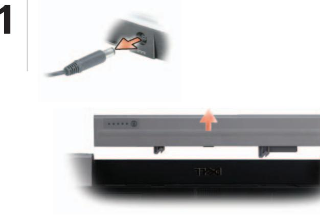
Disconnect the AC adapter and remove the battery.
